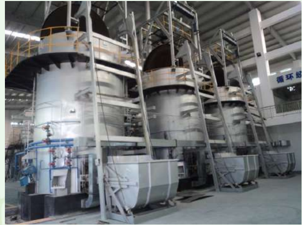
Figures above show Mechanical Grate Furnaces (daily capacity of 20 ton) which were built in 2014 for medical waste treatment in Zhanjiang.
