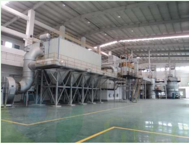
Figures above show Mechanical Grate Furnaces (daily capacity of 20 ton) which were built in 2014 for medical waste treatment in Zhanjiang.
